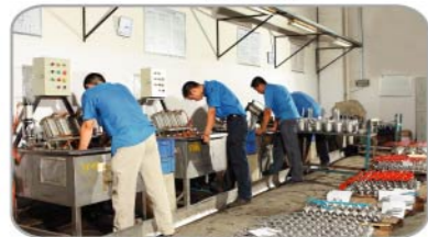
Pressure Testing 壓力測試
